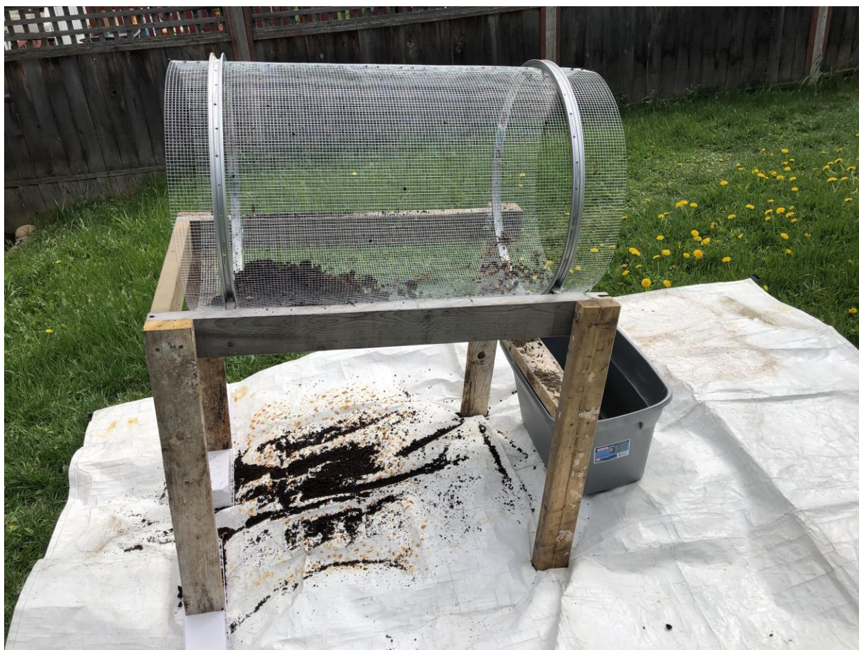
Figure 5: DIY trommel sifter for separating oversized pieces from finished compost.
