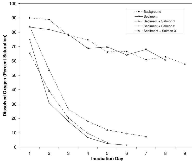
**Fig. 4** Biological oxygen demand curves for background, sediment, and the salmon and sediment samples ( $n = 3$ ). These data have been temperature corrected.
