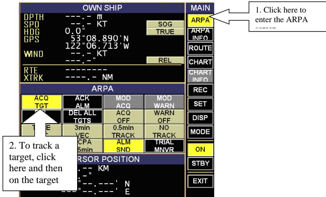
Figure 1. ARPA screen tracking buttons.
