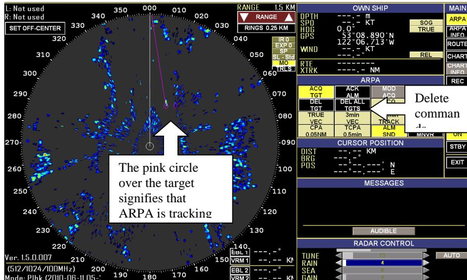
**Figure 2. Tracking in ARPA with Motion removal on.**
