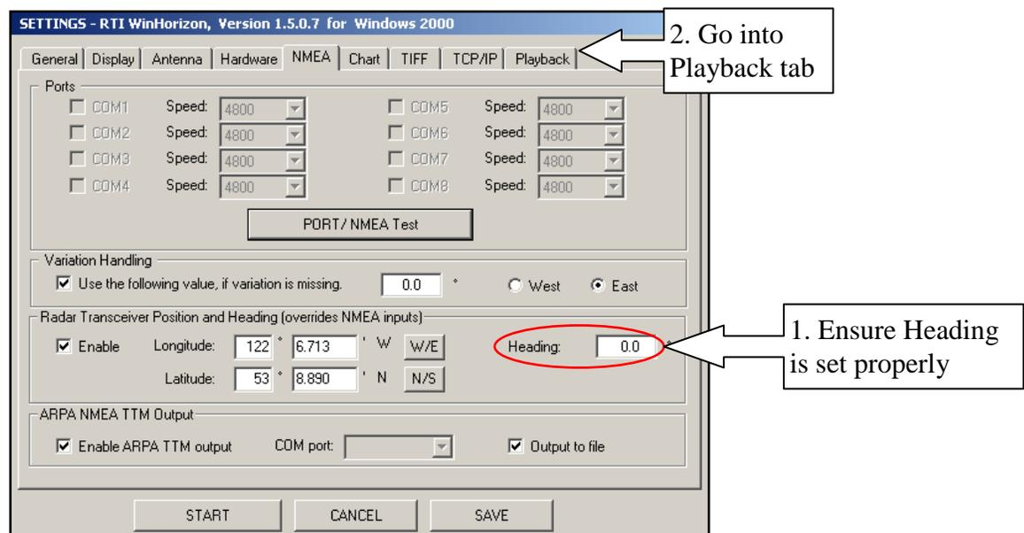
Figure 1. NMEA Tab if WinHorizon Set-up.
