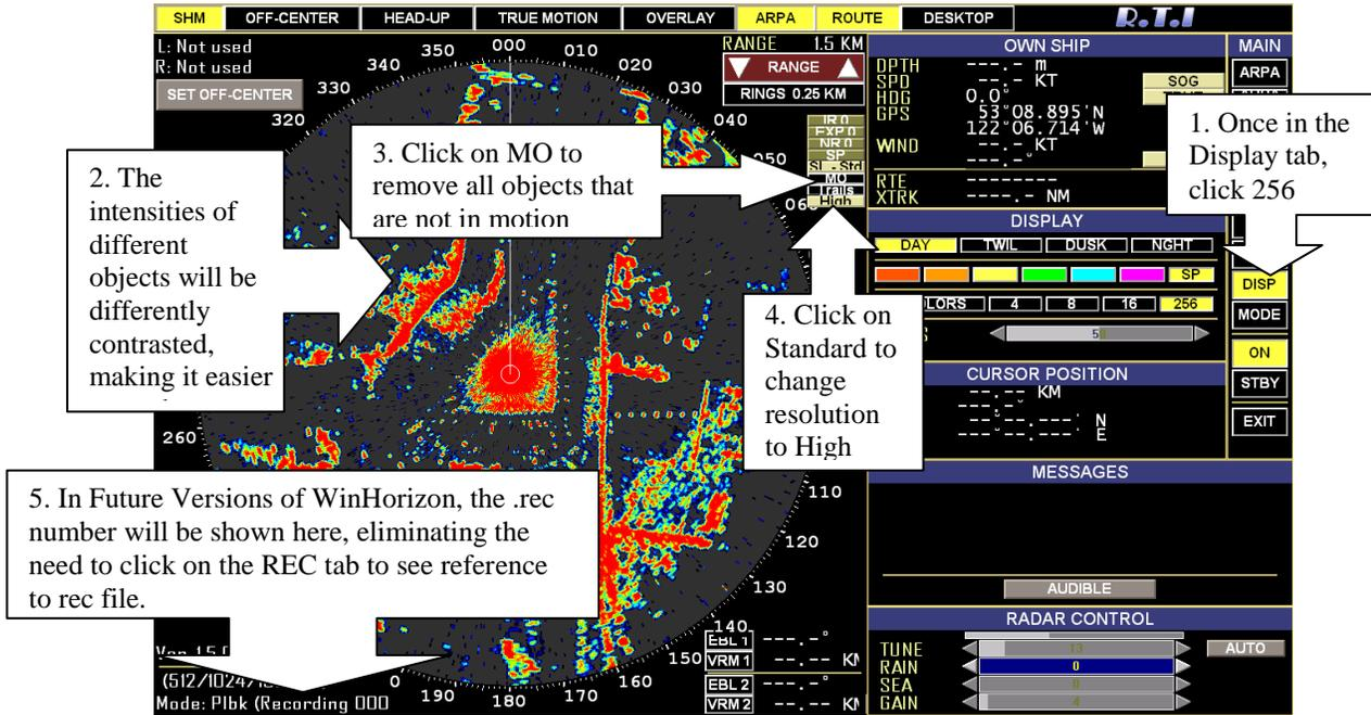
Figure 4. The WinHorizon Version 1.5.0.12 radar screen with 256 colours and high resolution.
