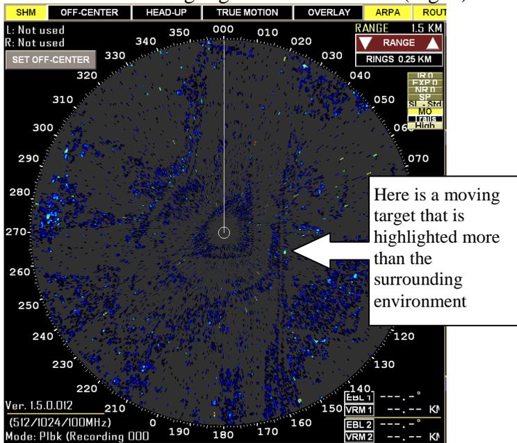
Figure 5. Image of WinHorizon Radar screen with Motion Removal on.
