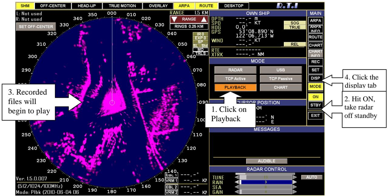
Figure 3. WinHorizon Playback for recording files.
