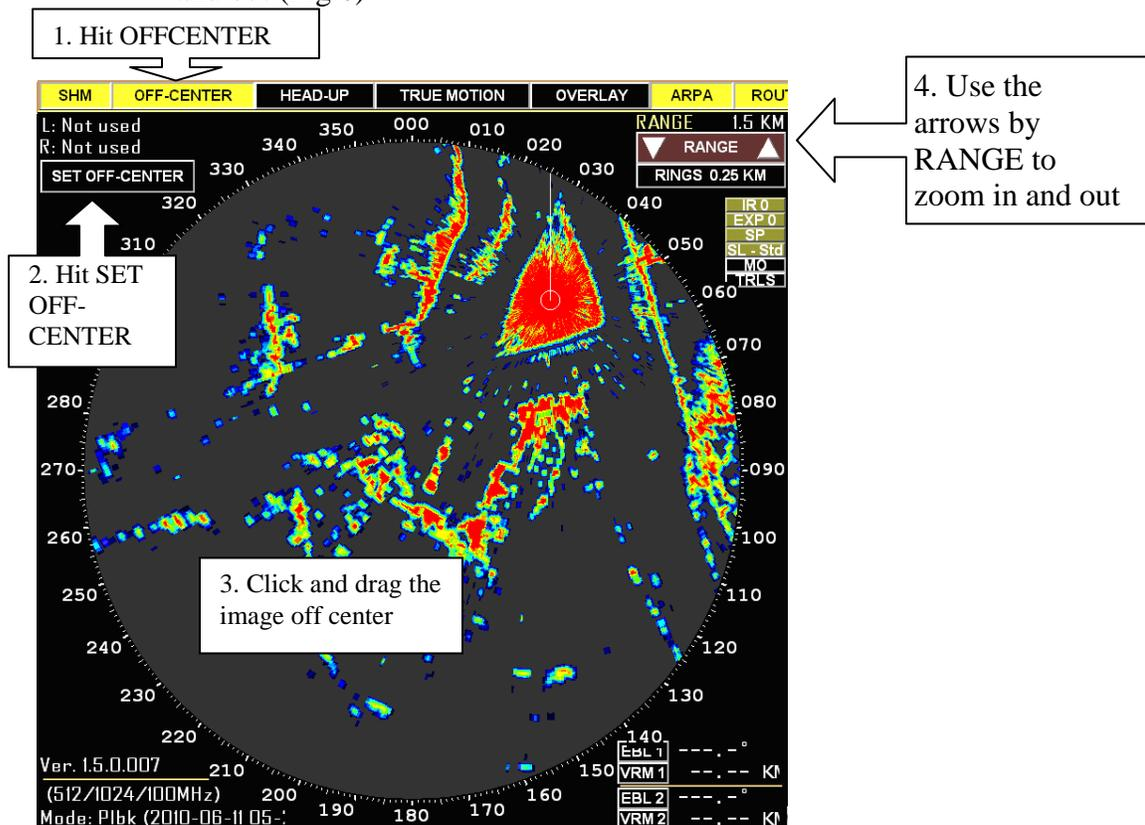
Figure 6. WinHorizon Radar screen set off center.
