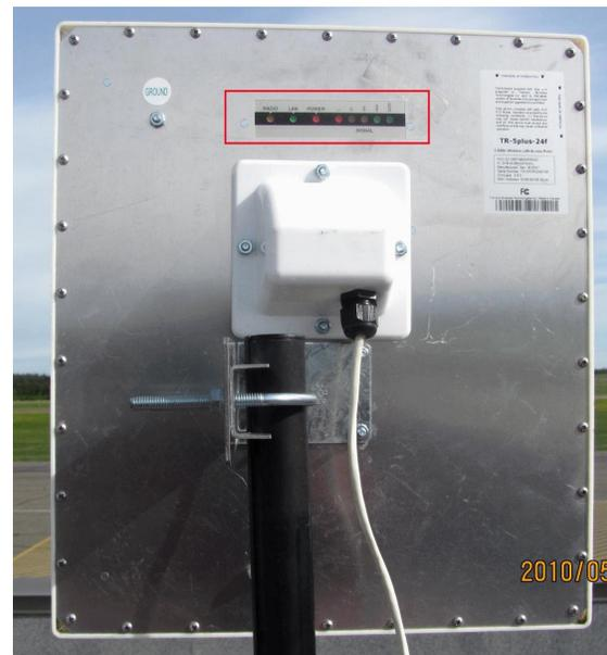
Figure 2. Receiver with a full signal (indicated by the green lights outlined in red)
