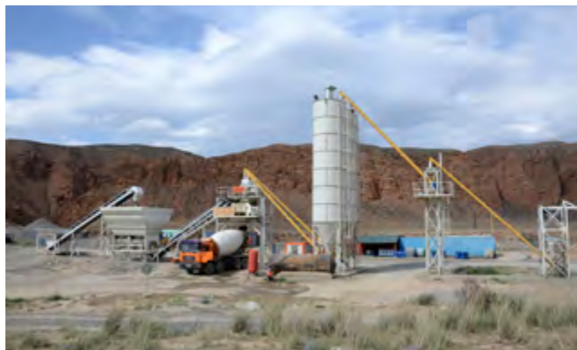
Cement batching plant in Naryn
