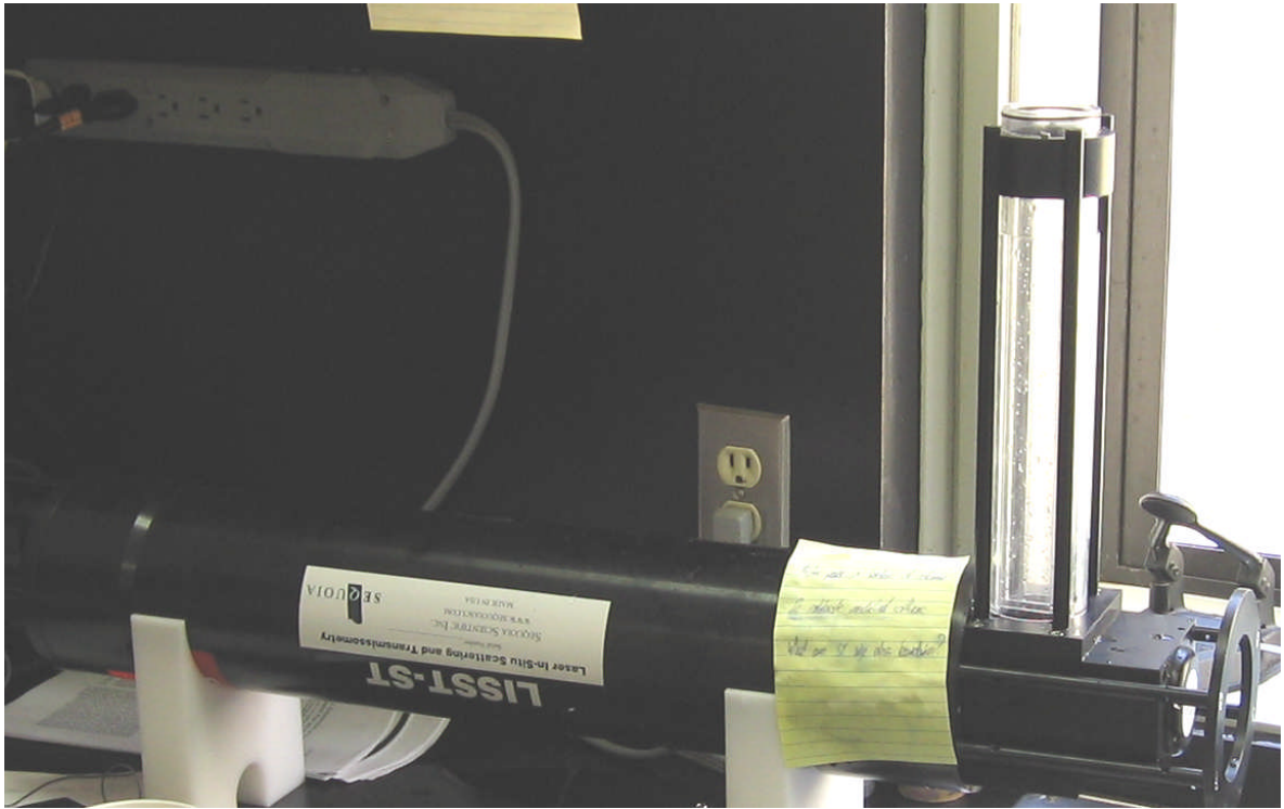
Figure 12: LISST-ST showing the 30 cm settling column and baffles (identified by water drops) prior to sample addition.
