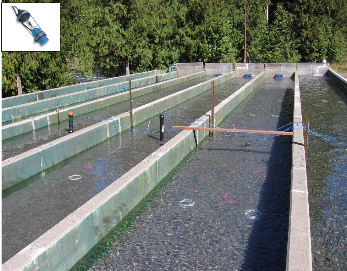
Figure 24: Upstream view of the flow-through channels showing the dissolved oxygen probe and down-pipes in the flumes along with the dissolved oxygen probe in the inset photo.
