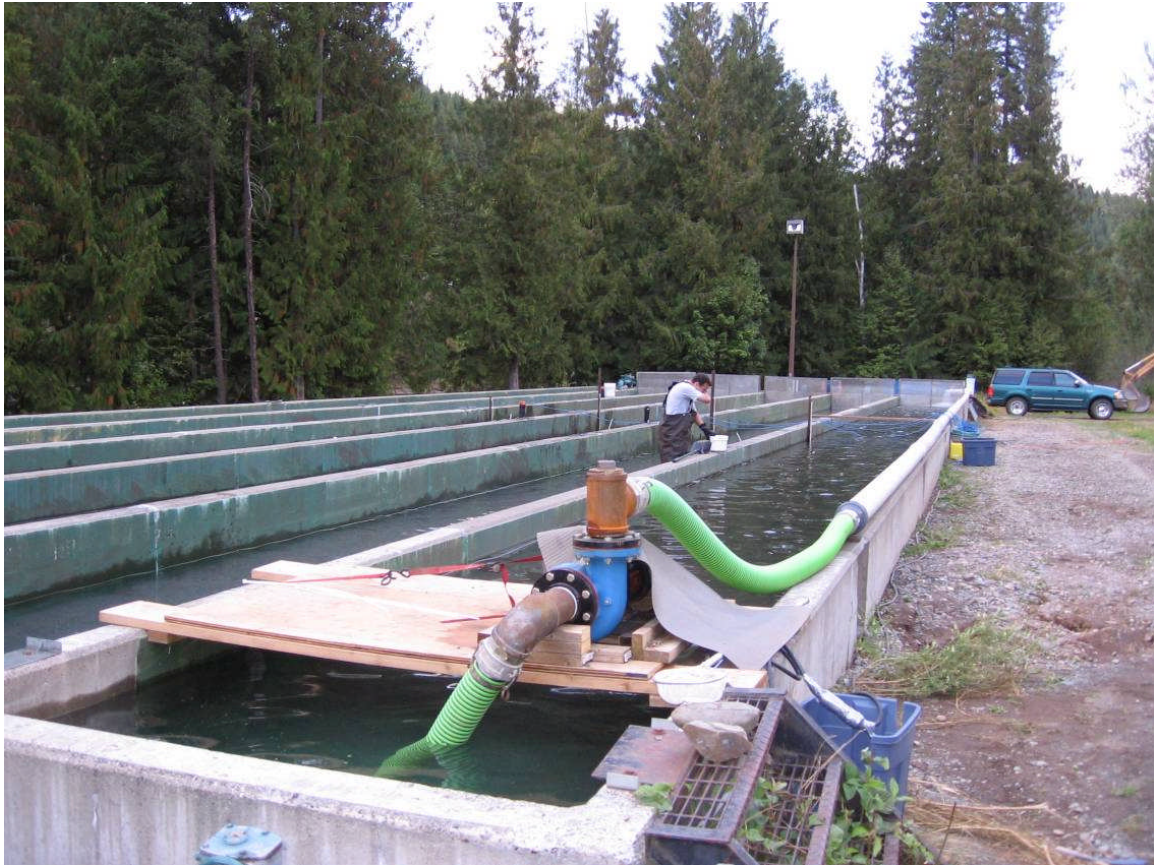
Figure 3: Upstream view of the re-circulating channel in 2006. In the foreground is the Gould's pump used to re-circulate water to the header tank. The LISST-ST was placed at mid-length of the channel near the staff gauge in the channel and Rubbermaid outside the channel. The flow-through flumes are to the left of the re-circulating one.
