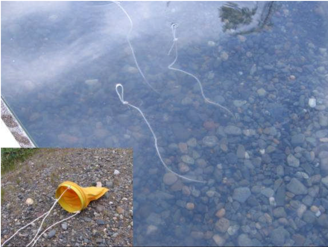
Figure 11: Infiltration bag deployed in a flow-through flume in 2007. Pull ropes extend from the flume's gravel surface and float in the water column for ease of location during their removal. Inset photo shows an infiltration bag lying horizontally on the ground prior to its installation in the channel – note the iron ring and the flexible waterproof bag (distance between ropes is ~20 cm).
