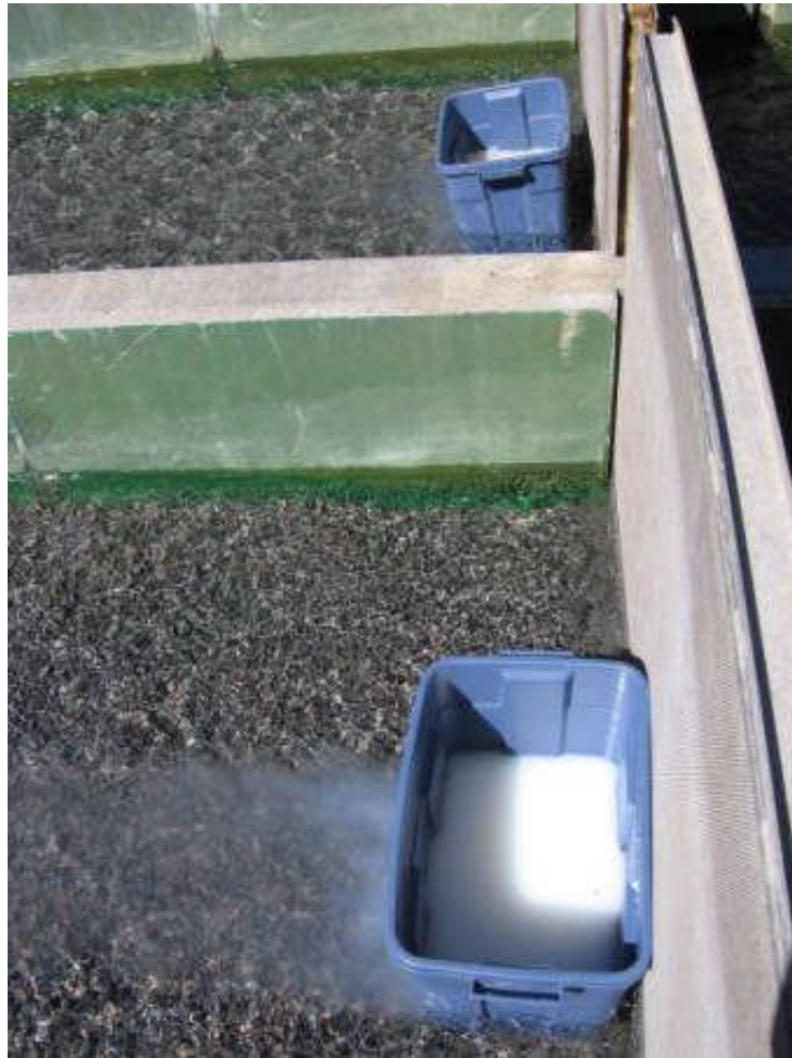
Figure 10: View of stock buckets in the flow-through channels. The clay treatment bucket is in the forefront and the salmon-clay mixture near the top of the photo. Note: water from the header tank passes through the turbulence baffle, enters the stock bucket on the right side of the photo, and then exits the stock bucket on the left as shown by clouds of clay (bottom) and salmon + clay (top).
