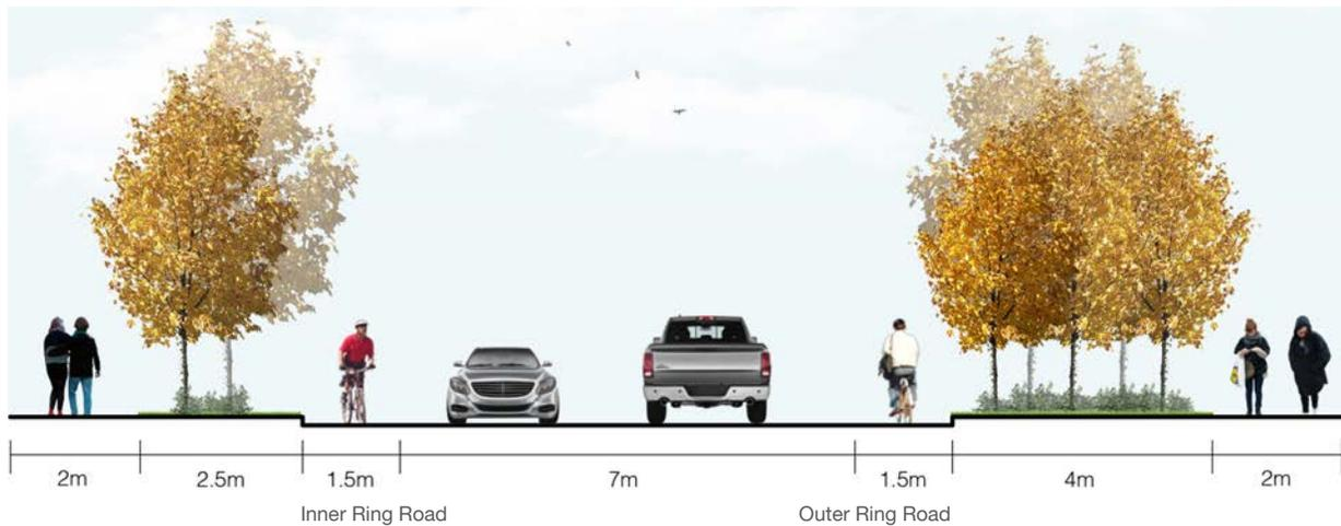
Figure 6.20 Typical Ring Road Section With Parking Bulge
