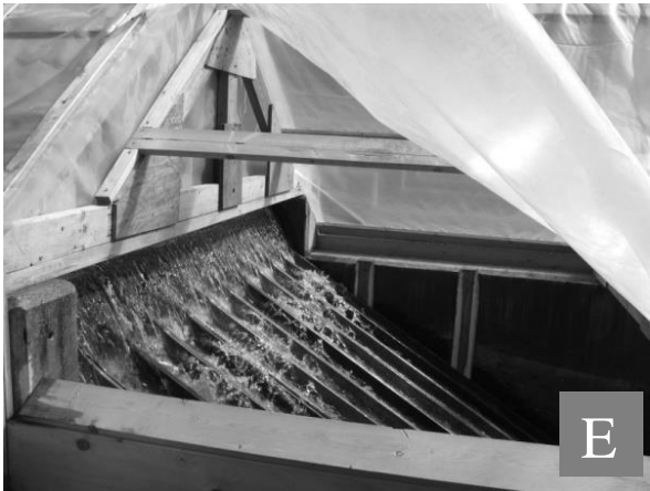
Figure 4. (a) Construction of flume roof, (b) Viewing window and frame, (c) Concrete wall removal and frame for viewing window, (d) Enclosed viewing platform, (e) Flow diffuser, and (f) Flume head tank.
