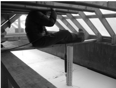
Figure 18. Use of Sontek 10-Mhz ADV to measure scour hole velocity under ice cover.
