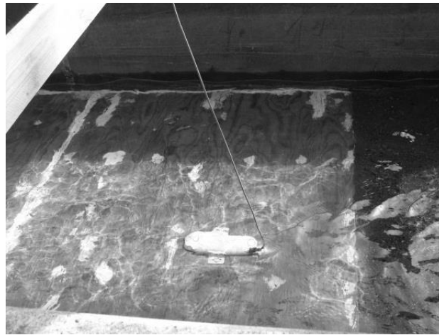
Figure 16. Sontek IQ mounted to flume floor.
