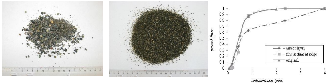
Figure 3.4- 6 Samples of armor layer, fine sediment ridge and related distribution curves
