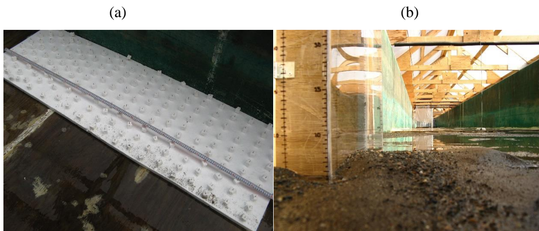
Figure 3.2- 2 (a) Inside view of the flume; (b) Rough ice cover used in the research
