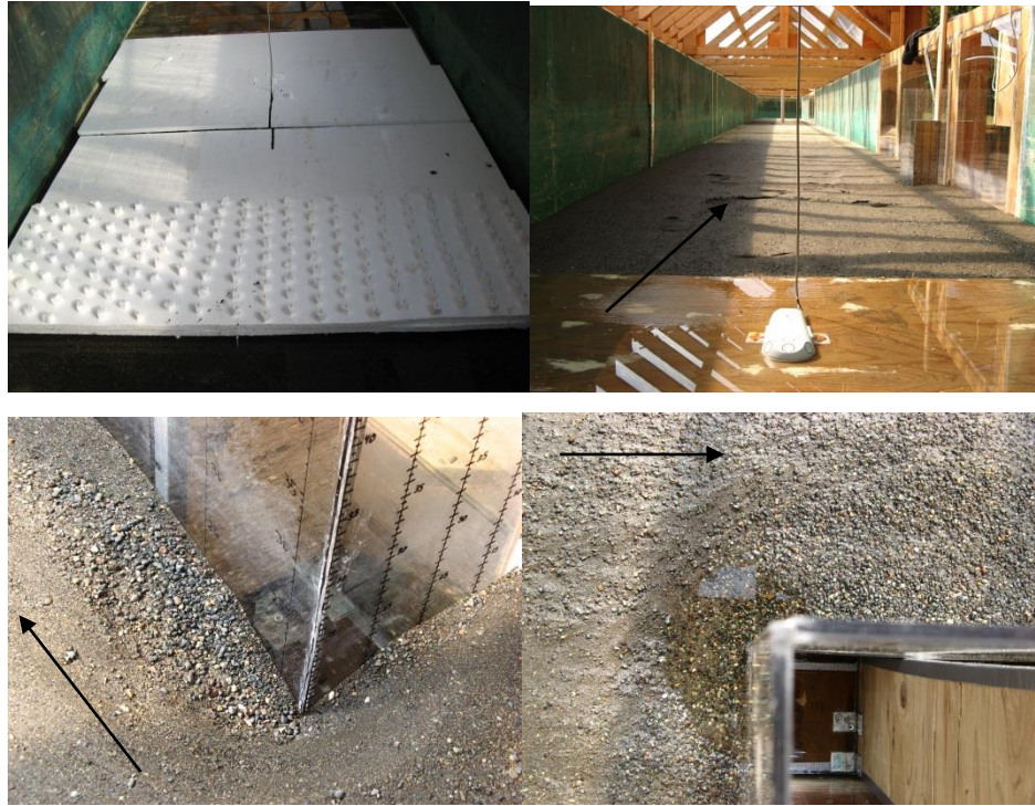
Figure 3.4- 3 Experimental flume set up and rough ice cover (up); Armor layer around the square abutment corner (bottom)
