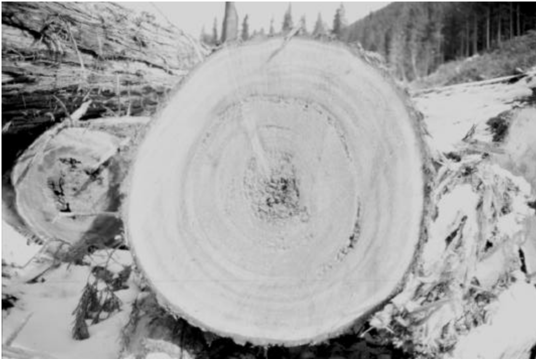
Figure 1. Pocket and ring rot in the but of western redcedar
