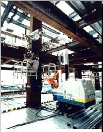
Welding robot installed with handling equipment
