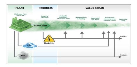
The current objective of this group is to explore the potential of developing a small, scalable bio-energy unit for smaller off-grid communities that would generate electricity, heat, and a range of tertiary opportunities for using both the energy and the 'waste' heat. The vision is to design the bio-energy unit for use with greenhouse operations.
